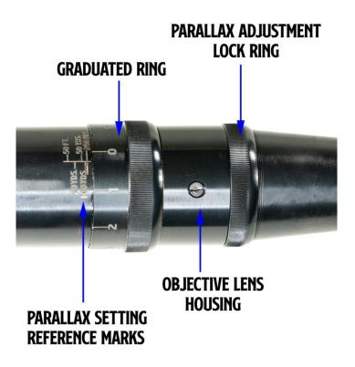
The following three steps are how to adjust the parallax setting: (1) Loosen the Parallax Adjustment Lock Ring
