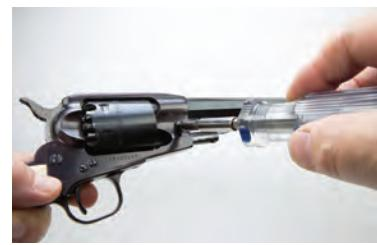
Both Ruger Old Army revolvers and Rogers & Spencer revolvers have base pins that are secured by a cross bolt. Use a screwdriver to turn the cross bolt to the unlocked position. (Right) With the cross bolt unlocked, the base pin can be pulled out to install the new cylinder.
