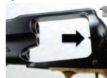
The revolver's hand, which is the little triangular piece sticking out of the frame blocks complete insertion of the new cylinder, unless you know the trick of getting by it.
