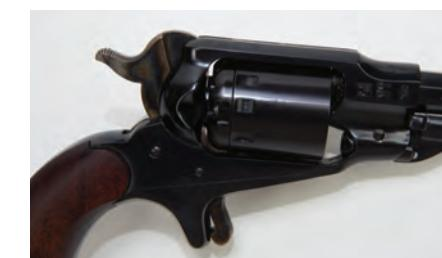
The 1863 Remington conversion cylinder has one extra bolt stop slot that allows you to lock up the revolver between chambers for safe carry.
