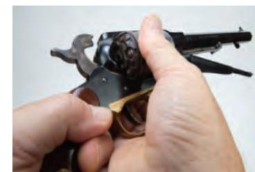
Insert the cartridge conversion cylinder from right to left. When you feel it hit the hand, keep pushing while rotating the cylinder clockwise. That rotation will lift the hand out of the way.
