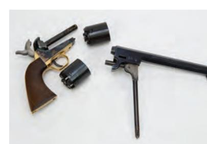
To replace the cylinder on Colt style revolvers, simply pop out the barrel wedge and remove the barrel assembly and the cylinder.
