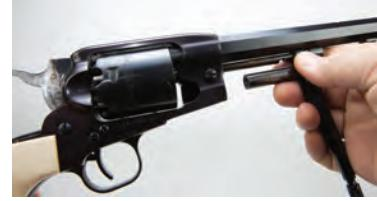
Next, hold the gun's grip with your right hand with the muzzle pointing away from you and in a safe direction, while you cup the gun's frame in your left hand. Your palm will be supporting the trigger guard and the forward part of the frame. Now you can use your left thumb to push the cap and ball cylinder out of the frame, into your waiting fingers.
