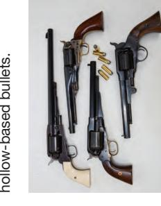
Cap and ball .44 caliber revolvers actually have .452-inch diameter bores. The proper cartridge conversion cylinders for these guns are chambered for .45 LC.
