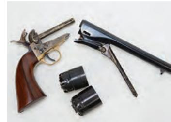
To replace the cylinder on Colt style revolvers, pop out the barrel wedge and remove the barrel assembly and the cylinder.
