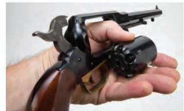
The cylinder can then be pushed out of the gun from left to right.
