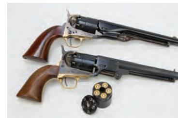
Taylor's & Co.'s five-shot, .45 Colt cylinders fit both 1860 Army revolvers (top) and .44 caliber 1851 Navy revolvers (bottom).
