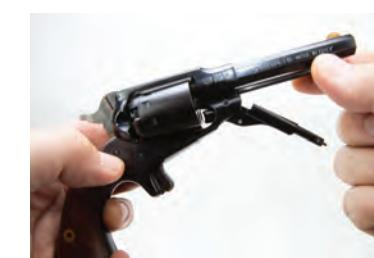
To install a conversion cylinder in the 1863 Remington place the hammer on half-cock, drop the loading lever and pull out the base pin.
