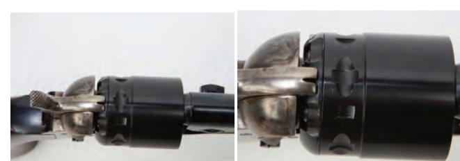
The cylinder bolt-stop slots allow you to lock up the cylinder with the hammer lowered between chambers for safe carry. The bolt slots between the chambers have half-moon shaped leads/ramps on each side of the slot. The slots for the chambers have no half-moon shaped leads.
