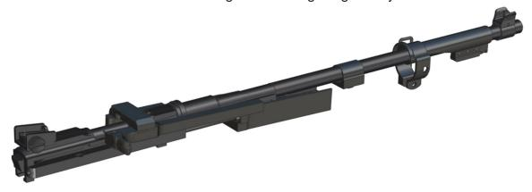
3. Pull back the lever until it reaches an intermediate position. In this position, if you push down the lever, the guides of the lever can be released from the guides of the receiver # 36
