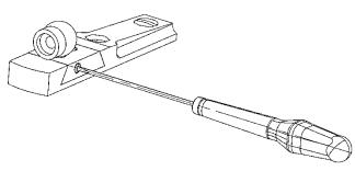
**Elevation** is adjusted by loosening the lock screw on the left hand side and turning the aperture stem up or down on its threads, then locking it in place with the screw.
