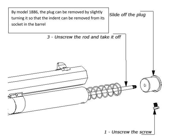
When the rod has been removed, replace the plug in its seat. In the Take Down version there are two screws to disassemble.
