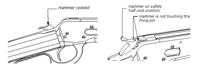
Hammer in safety position is strictly recommended when firing is not imminent and cartridge is chambered.
