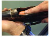
It's important that, prior to closing the lever, you should hold the barrel with the mouth facing slightly downwards and at the same time you should rotate the receiver about 20° on the left side as shown in the picture.
